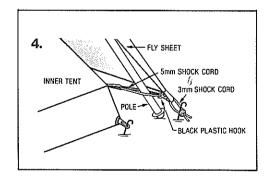
This system of using one peg for two guy points has the advantage that you have fewer pegging points to find and less weight/bulk in the packed tent. In some cases, particularly uneven ground, you will find the tent pitches more neatly if separate pegs are used for the 5mm and 3mm shock-cords.
